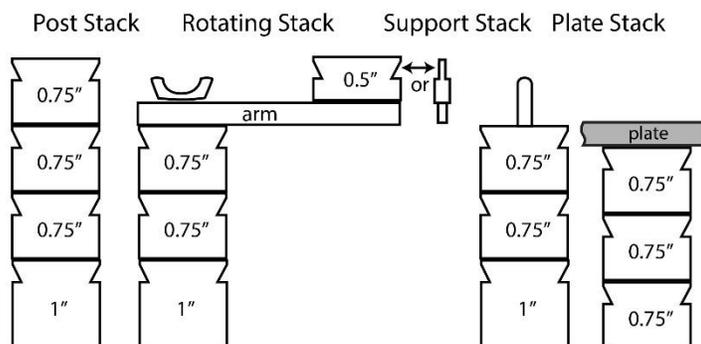
The Universal Fixture plate that makes up the support bed for the Access DH Prober has threaded mounting holes spaced at 2 inch intervals for attaching the Post, Rotating, Support and Plate stacks.
