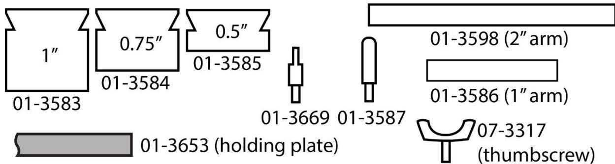
The kits pieces can be used to create a “Post Stack” which serves as an anchor support from the board edge, an adjustable “Rotating Stack” that supports the PCB from the board edge, a “Support Stack” which supports the PCB from underneath and a “Plate Stack” which uses a secondary holding plate. Use the diagrams shown on the following pages of this document to create stacks used with the Top, Middle, Bottom and Base slots of the Access DH Prober.
